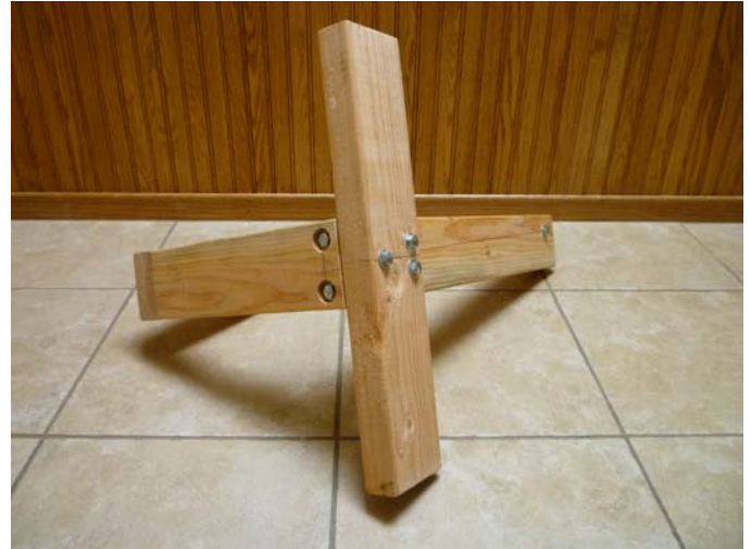
Bottom side of stand. Care should be taken so that none of the five attachment bolts conflict with one another.
