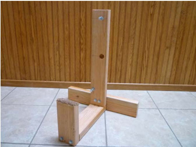
Newly constructed bell housing stand.
