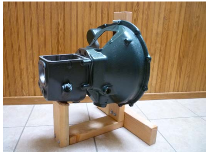
Mounted bell housing with transmission housing attached.
