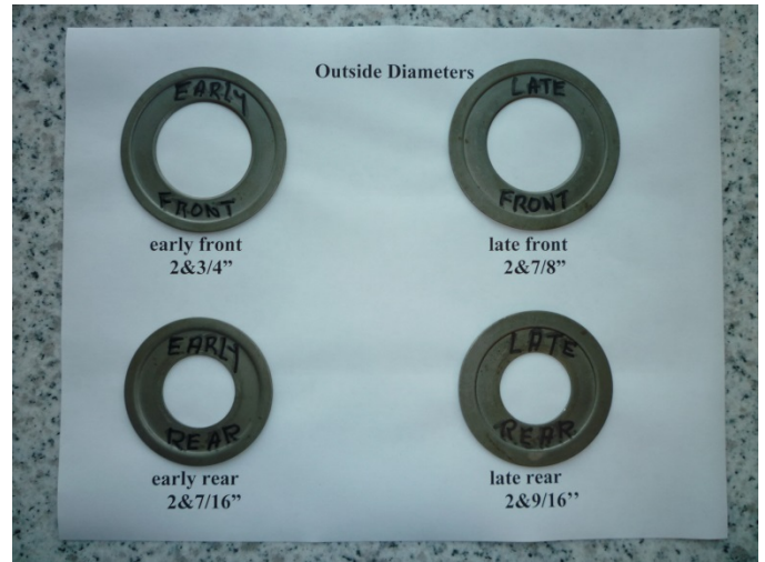
The early and late oil baffles are shown here. The outside diameters of the late baffles were increased by 1/8" over the early baffles.
