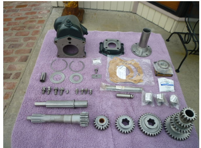
A complete transmission parts layout. Note the two baffles and snap rings directly in front of a late housing
