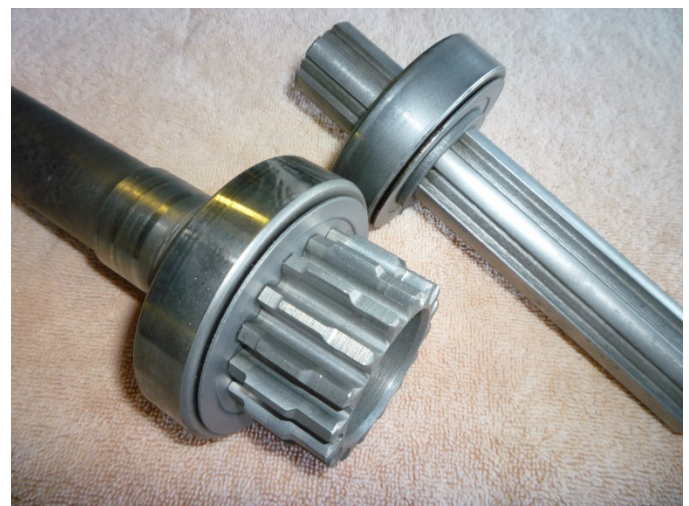
The off-set on the baffle should produce a nominal 1/16" space around the outside diameter and not touch the bearing.
