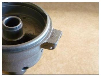
The 1931 distributor has a bridge across the area where the two cap clamps attach.
