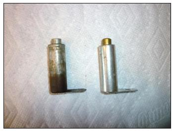
An earlier condenser on the left removed from a distributor core measures 2&1/32" in overall length. The condenser on the right recently purchased measures 2&1/8 in overall length.
