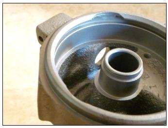
The 1931 casting is more robust. Note the protrusion on the left side of the window where the lower plate tab and the fiber washer at the end of the condenser reside. This is where the tab on the lower plate can short out with an extralong condenser.
