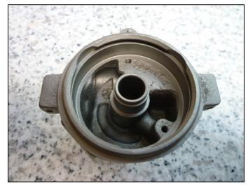
A common problem found with many distributor cores is that the attach points for the cap clamps is broken off. This damage does not usually occur when the distributor is in service on the car. It occurs when removed and someone drops it on the ground. Bridging the clamp attachment added extra strength.
