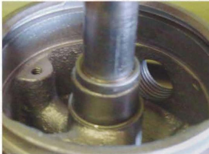
The distributor housing is turned over under the press and the insertion tool is inserted from the top and the bushing is pressed back into place if it slightly overran the top of the shaft tunnel.
