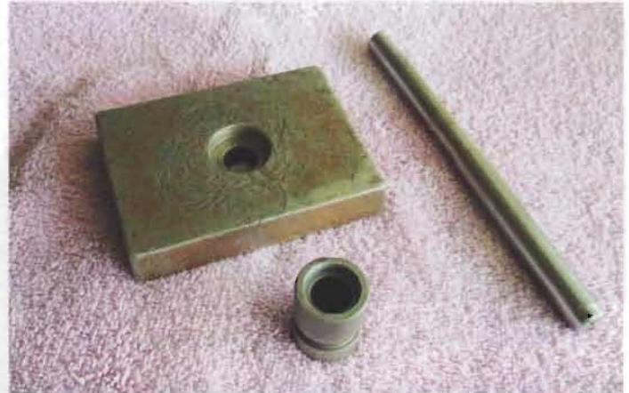
The three tools used to press in the new bushings. The plate is at the upper left, the collar is at the lower center, and the insertion tool is on the right.
