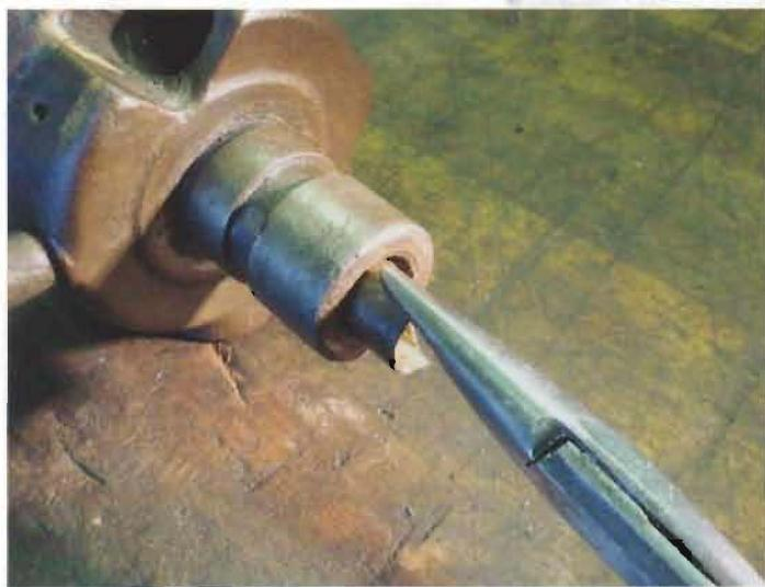
The bottom bushing is curled out with long nose pliers.
