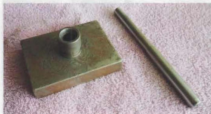
The collar is placed inside the recess in the plate.
