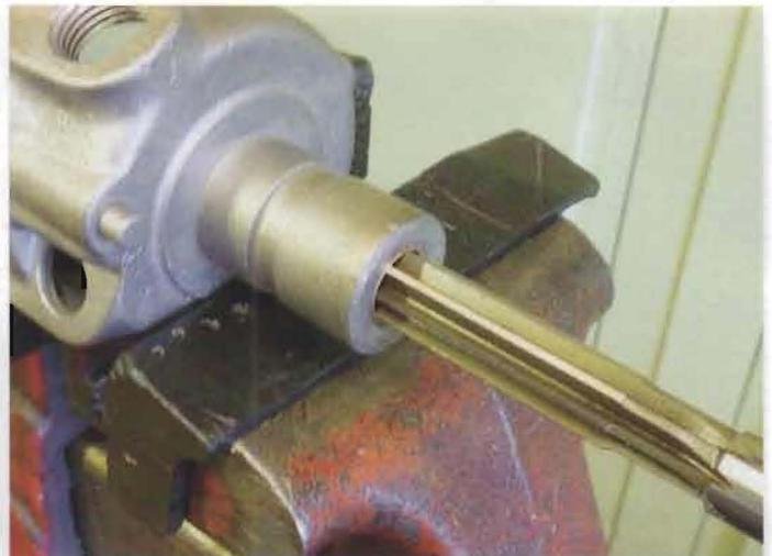
With both bushings installed, and with no cracks in the housing, the two bushings are reamed to accept the new shaft.
