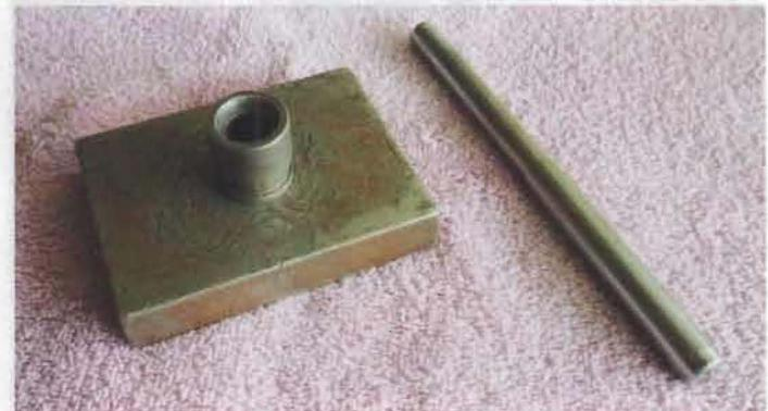
The collar is placed inside the recess in the plate.
