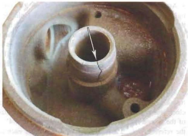
Typical crack found near the top bushing.
