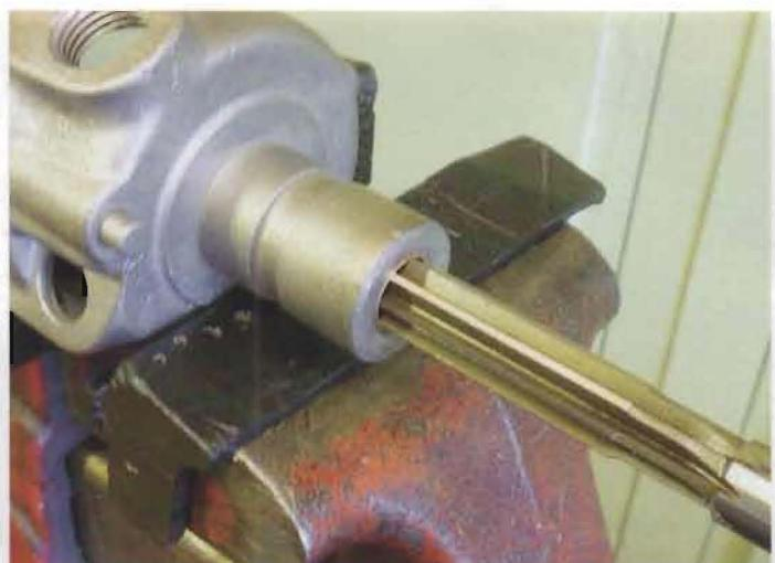
With both bushings installed, and with no cracks in the housing, the two bushings are reamed to accept the new shaft.
