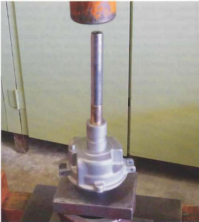
The distributor housing is placed under the press upside-down on the collar and on the plate. The top bushing is inserted from the bottom.
