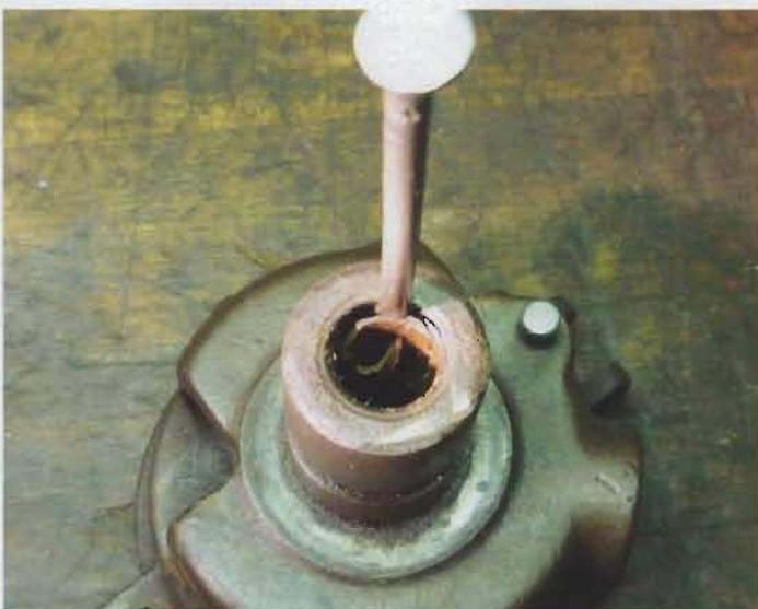
Both bushings in the distributor housing have been split with a hacksaw blade and the modified nail is gently tapped down along the split.
