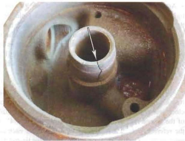
Typical crack found near the top bushing.
