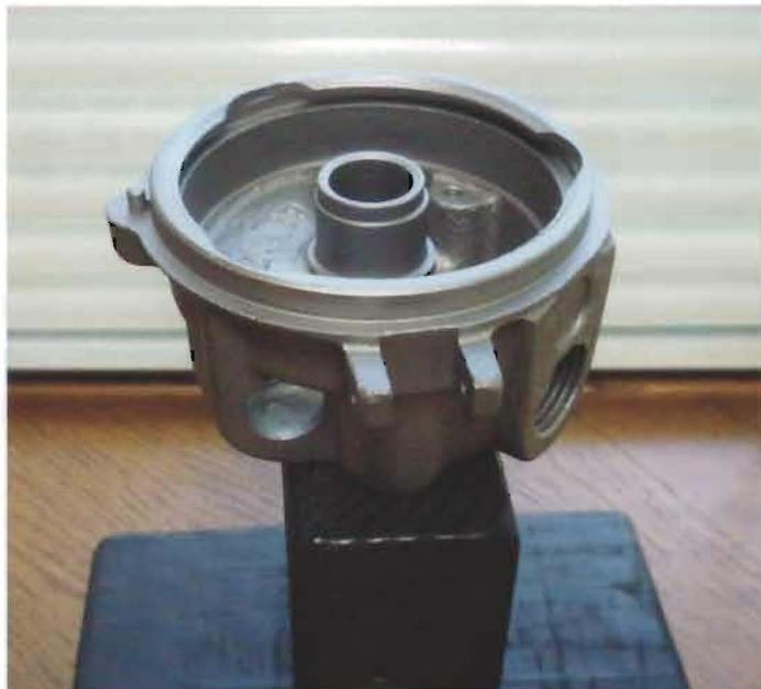
Bushings have been removed, the housing has been de-greased and bead blasted and is ready for the installation of two new bushings.
