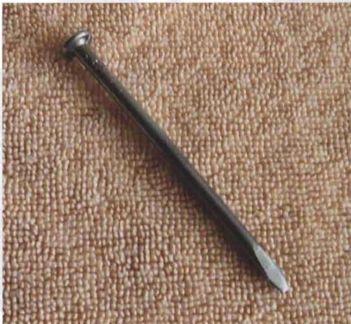
Common nail shaped to a chisel point.
