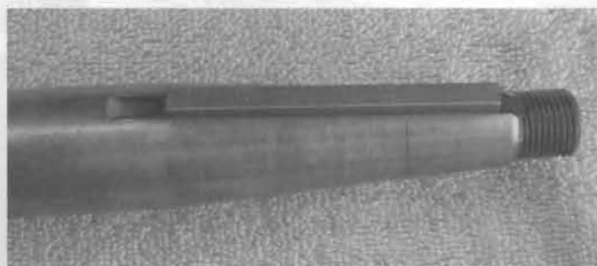
Drive shaft used with the later style pinion gear.
