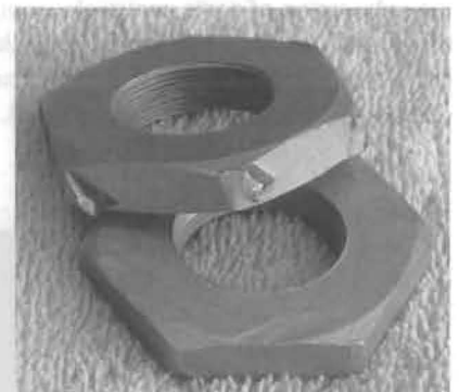
Early chisel molested pinion nuts.
