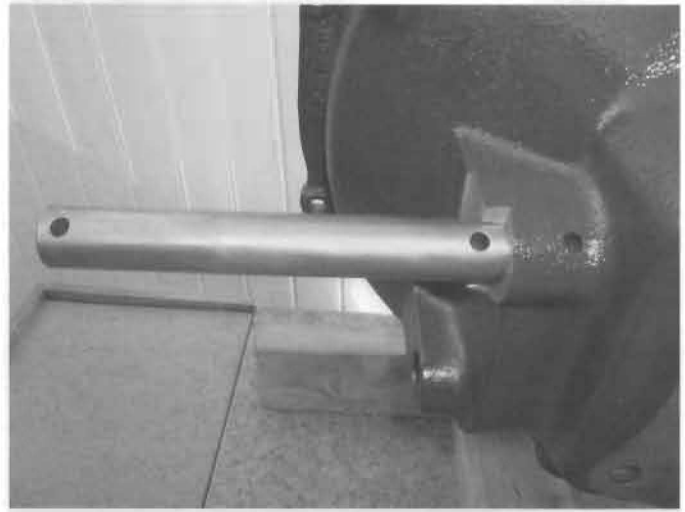
The end of the pedal shaft with the pin hole about an inch from the end of the shaft goes into the bell housing. The other end of the shaft has the hole close to the end of the shaft. Accurately line up the hole in the shaft with the hole in the bell housing before driving it in.
