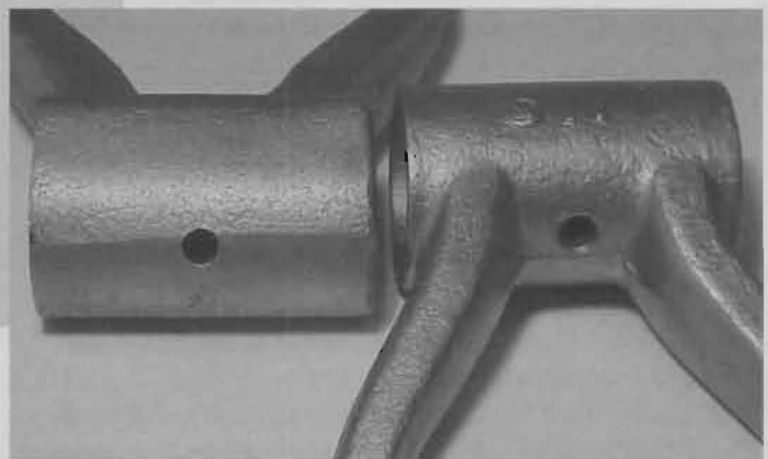
The above photo shows two A7515-B forks with the original 3/16" holes. Note there is ample material to drill the holes out to 5/16".
