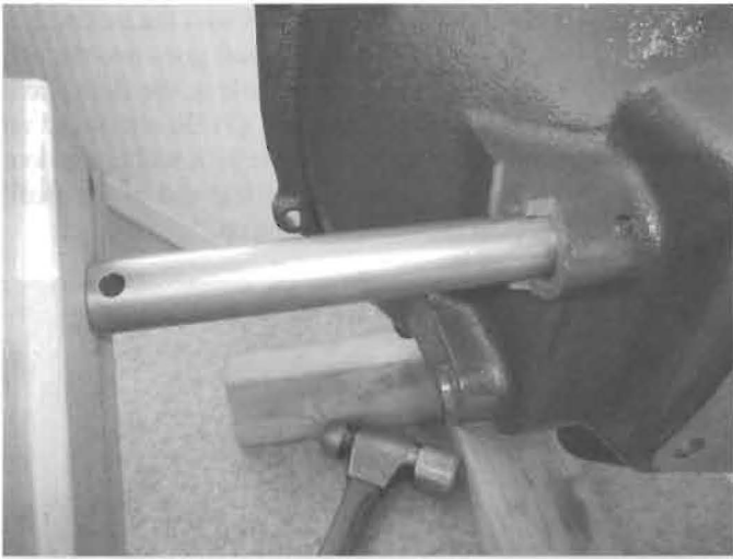
Use a block of wood so as not to mushroom the end of the shaft with the hammer.
