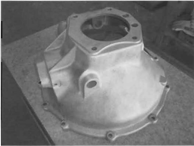
The outside of the bell housing after it was de-greased and bead blasted.
