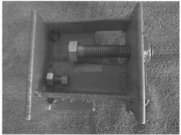
Crude but effective tool used to push out a stubborn pedal shaft. The tool is bolted at the bottom to the four transmission mounting holes in the bell housing. The large bolt is turned with a wrench to push the shaft out.
