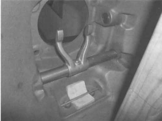
Yoke oriented correctly on new clutch release shaft. Radius rod bolt heads and felt installed correctly and retained by the long pin.
