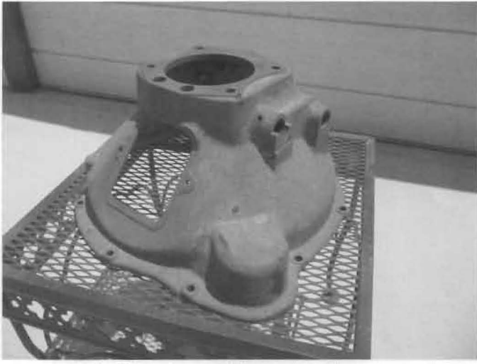
Disassembled bell housing ready for bead blasting and painting.
