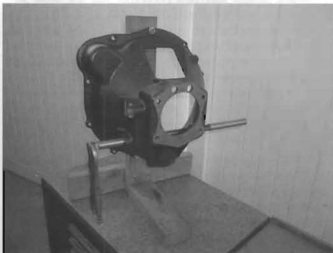
This bushing reamer is long enough to fit through both bushings at the same time to ensure they will line up with each other.
