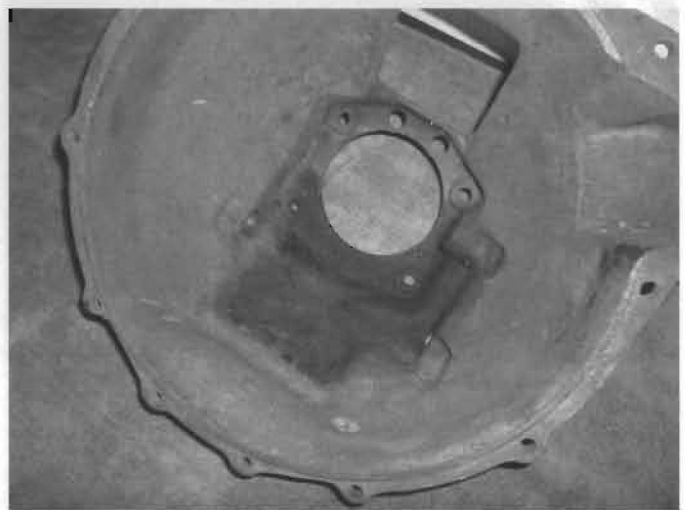
The inside of a bell housing can be extremely cruddy. This one will have to be de-greased before it can be bead blasted.
