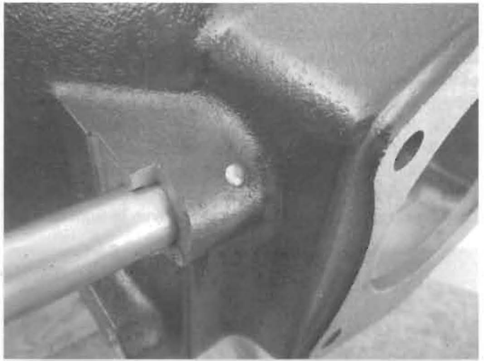
Drive the pin in until it is flush with the housing.
