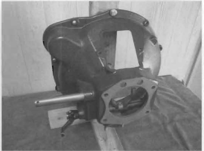
Complete restored bell housing. New clutch release shaft, bushings, and pedal shaft have been installed. The bell housing is ready for installation in the car once the transmission has been attached.
