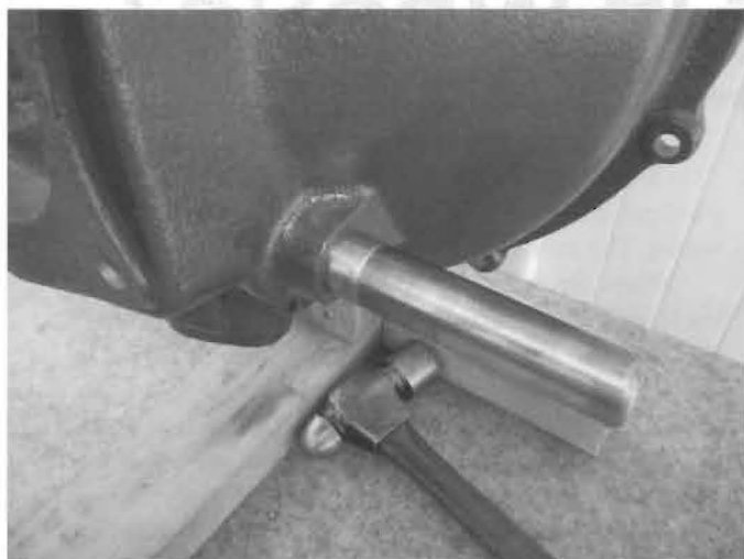
New bushings are driven in with a bushing tool.
