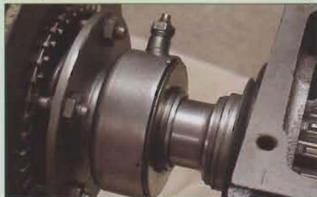
Throw-out bearing and extra oil baffle
