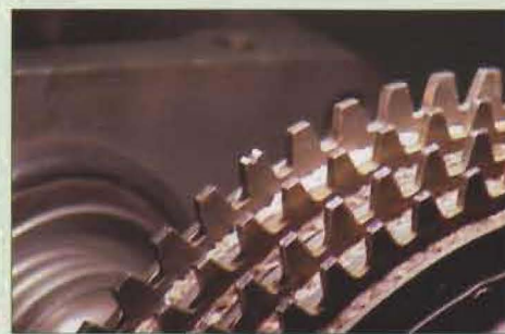
The notched tooth driving disk
