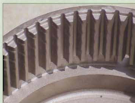
Notches worn in the flywheel
