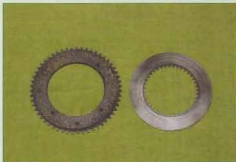
Driving disk (left) driven disk (right)
