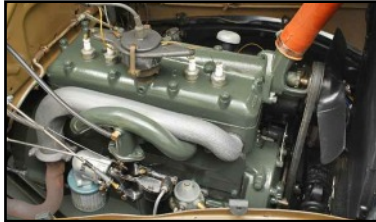
Model B engine can be identified by the fuel pump on right side of block and no oil drain tube.
