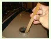
Tools for adjusting the float arm are simple: a piece of coat hanger wire and a paint stir stick. If you have the original spark arrester in your tank, it will have to be removed. Use the bent wire to pull up the float arm (through the gas fill-hole). When the float hits the top of the tank, the gauge should read "F" full). Use the paint stick to push the float arm to the bottom of the tank. The gauge should read "O" (empty).
